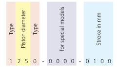
Example: Article number for a ZS cylinder with a diameter of 25 mm, standard connection and a stroke of 100 mm
